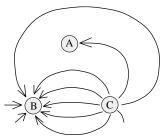
resistors is the same, the circuit can be re-drawn as shown to the right. Being a parallel combination, the equivalent resistance is 5  $\Omega$ . This response is true. Are there other possibilities?]
